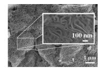
Templation in liquid ammonia: The first porous materials formed by templating in liquid ammonia utilize the liquid-crystalline phase formed by cellulose/NH<sub>4</sub>SCN in NH<sub>3</sub>. By changing the proportions of reactants, the porosity, surface area, and morphology of the materials can be modified. The as-synthesized mesoporous materials present a lamellar morphology (see picture).
