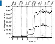
The importance of the oxide:  $Ce_{0.8}Ni_{0.2}O_{2-y}$  is an excellent catalyst for ethanol steam reforming (see graph). Metal—oxide interactions perturb the electronic properties of the small particles of metallic nickel present in the catalyst under the reaction conditions and thus suppress any methanation activity. The nickel embedded in ceria induces the formation of O vacancies, which facilitate cleavage of the O—H bonds in ethanol and water.
