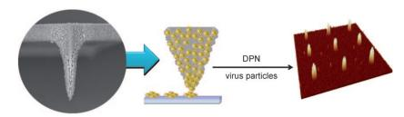
**Pen-pushing**: Direct-write dip-pen nanolithography (DPN) using a tip coated with nanoporous poly(2-methyl-2-oxazoline) allows the creation of precise patterns of large-sized biomaterials such as viruses.
