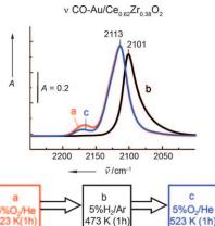
Strong and reversible modification of the chemical properties of supported Au nanoparticles caused by alternating oxidizing (a and c) and reducing (b) pretreatment of  $Au/CeO_2$ – $ZrO_2$  catalysts were revealed by a methodology that combines FTIR spectroscopy (see picture), studies on the volumetric adsorption of CO and ultimate oxygen storage capacity, determination of metal dispersion by electron microscopy, and X-ray photoelectron spectroscopy.
