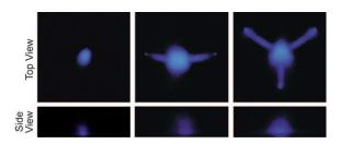
It's the pits: Increased efficiency and controllability of sonochemical reactions was achieved with silicon surfaces on which pits were micromachined to entrap gas, which, upon ultrasonic excitation,
