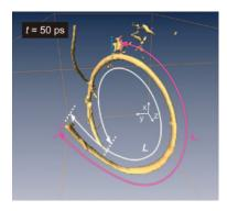
Time and motion studies: 4D electron tomography enables the direct investigation of transient states of materials, structural dynamics of large molecular objects (for example the motion of a spiral carbon nanotube), and biological systems under controlled conditions.
